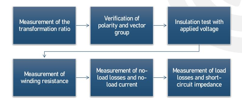
The test results are recorded and stored in a dedicated register. The register is used to monitor the quality of transformers and to identify any issues that may arise in the future.
